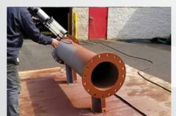
For larger surfaces, application time can be dramatically reduced with the **MeCaSpray Gun**. The MeCaSpray equipment can be used with the following cartridges:
